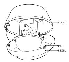
Figure 4. Lower Dome and Bezel Installation
